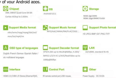
USB keyboard cable port, 2.4GHz air
