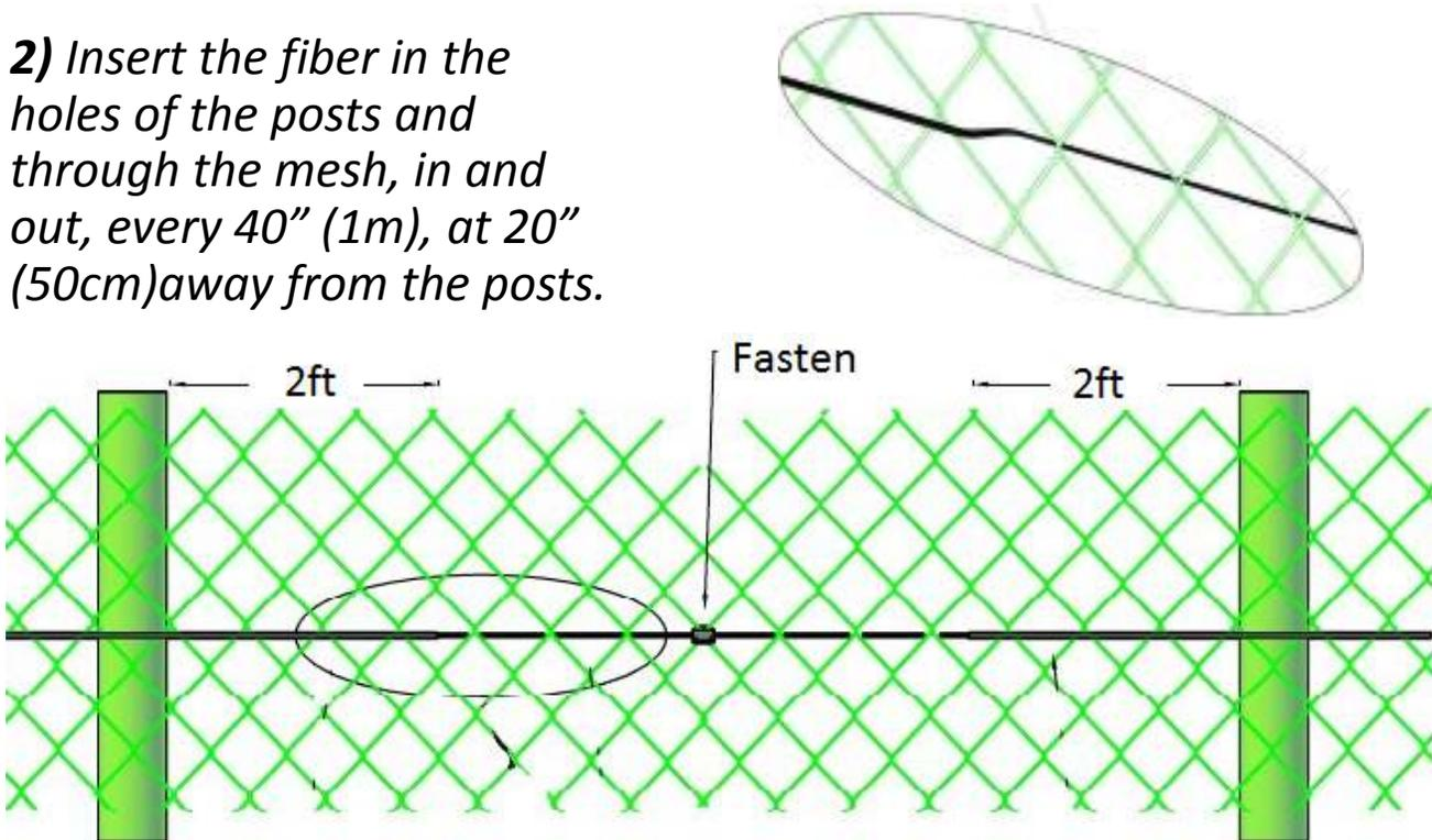
*Tie the fiber to the mesh only once in the middle between the two posts, as shown in the figure beside:*
