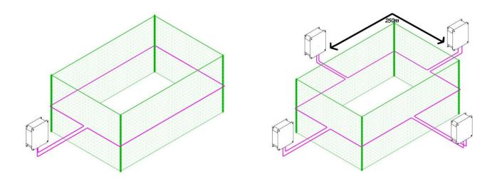
When installing on a fence with no mid support beams.
