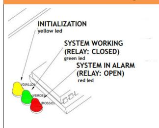
11) 4- Connect the alarm relay (10A to 240VAC) to the alarm system; you can place the anti-tampering sensor in-series.
